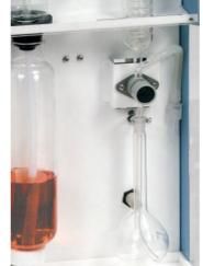
Automatic termination of final distillation at 200 ml of distillate. By using the ADD function small quantities of distillate can be added to accurately fill the matrix flask to the mark without having to add water to the distillation.
